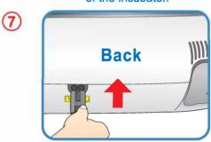
Insert the power cord in the socket at the back of the main body.
