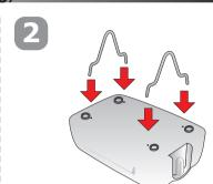
▶ Please put the Egg-Turning wires in the holes, bottom outside of the main body.
